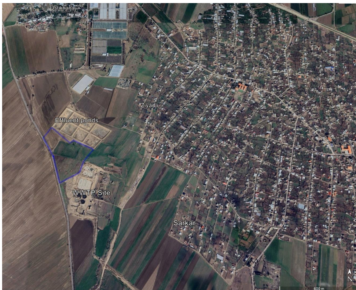
Figure 2. The sites of the WWTP and effluent ponds, and a proposed location of additional land (blue contour) that may be procured for sludge management, if agricultural re-use is not feasible
